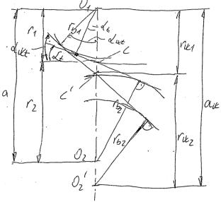
$$r_{b_1} = r_{w_1} \cos \alpha_{wt} = r_1 \cos \alpha_t$$
